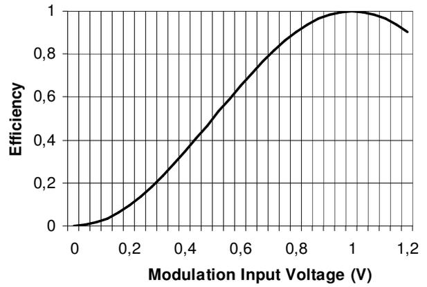
**Typ AO effic vs Wavelength 488nm driven**
